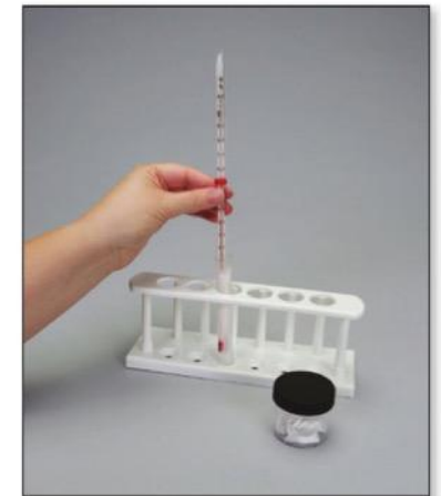
Figure 1.6 Make sure you wait about 30 seconds after placing the thermometer in the test tube of water before you read the temperature.
