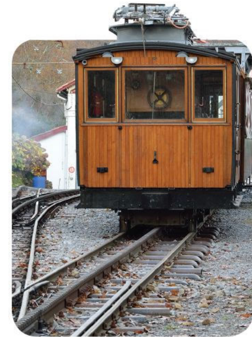
Cog railway system
